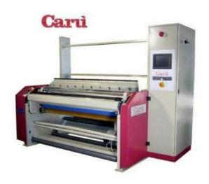
MAIN FEATURES: This machine has been design to cut the corduroy ribs;
